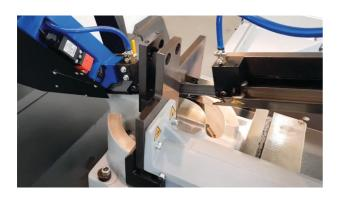
ARG 235 Plus Band saw machine can cut materials up to 235mm in diameter, featuring a sturdy cast iron frame that reduces vibration and enhances durability. Equipped with a three-phase, dual-speed motor (40 and 80 rpm), this machine enables precise cutting of various materials including stainless steel and tool steel.
